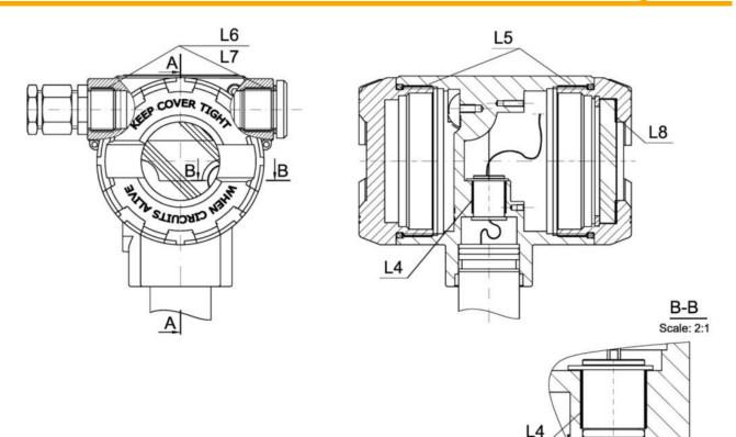
Figure 8. Flameproof joints of enclosure.
