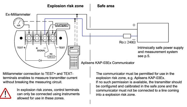
Figure 5. Connecting Exi transmitters and probes
