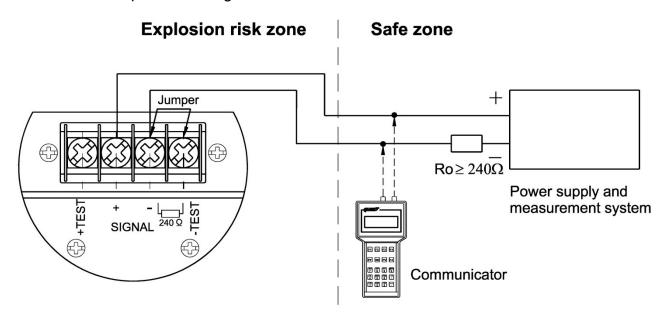
Figure 6. Connecting Exd transmitters and probes
