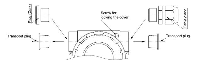
Figure 7. Installation of cable entries and blinding plugs
