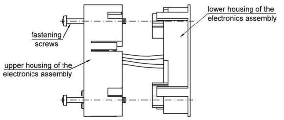
Figure 8. View of disassembled display unit
