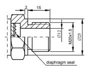
Fig.6a. P-type connector with M20x1.5 thread
