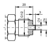
Fig.8a. G1/2-type connector with G1/2" thread
