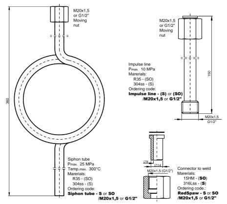
Fig.3. Additional equipment for fitting of pressure transmitters.
