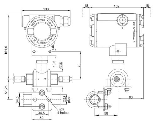
Assembly Kit ("Mounting bracket  $\varnothing$ 25" made by APLISENS) for fitting differential pressure transmitters with P-type connector on a  $\varnothing$ 25 pipe see catalogue cards "Fitting accessories".
