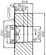
Fig.8d. Weldable fitting ring for use with transmitters with CG1/2 - type connector Material – 316Lss
