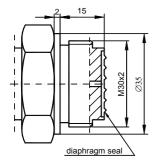
Fig.7a. CM30x2-type connector with flush diaphragm with M30x2 thread,
