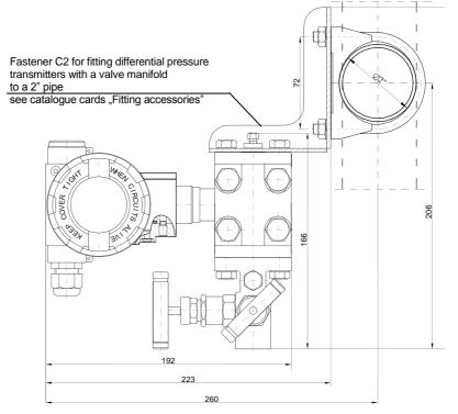
Fig.13. Example: how to install the APR-2000... transmitter with a valve manifold to a 2" pipe.
