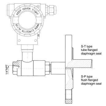
Fig.10. APR-2000... differential pressure transmitter with a single direct diaphragm seal (example).
