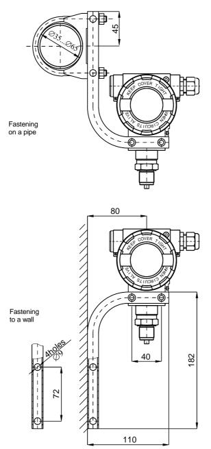
Fig.4. Example: how to install the APC-2000...
