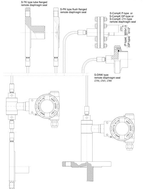
Fig.14. APR-2200... differential pressure transmitter with two remote diaphragm seals(examples).
