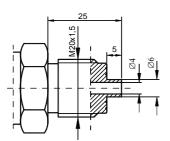
Fig.5a. M-type connector with M20x1.5 thread
