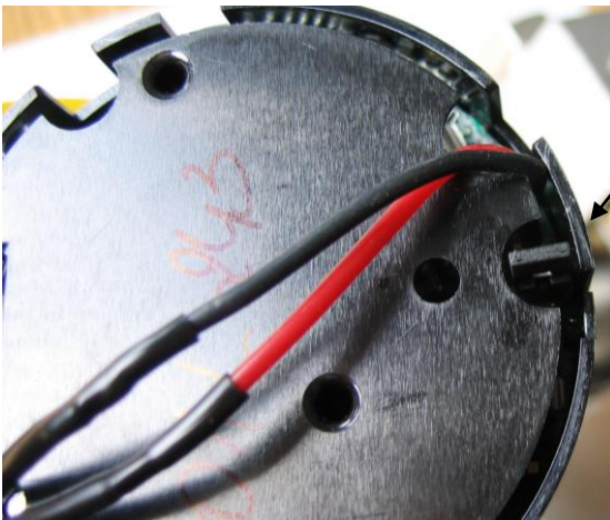
Fig. 5. Back lighting jumper view at transmitter electric board - only for version "MID" (unit display back side).
